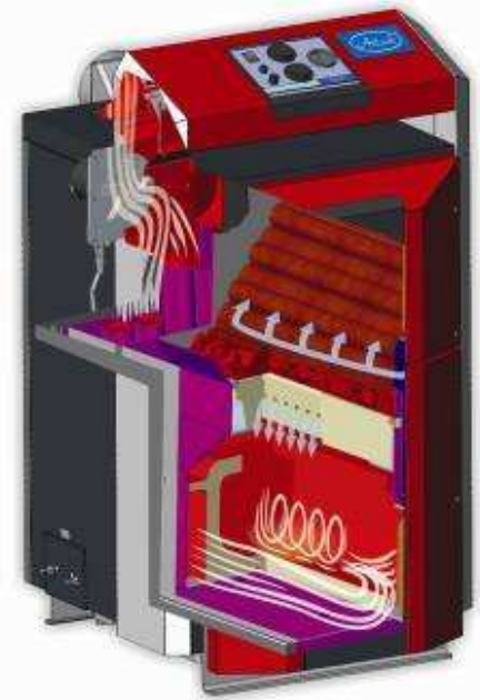
DPX Boiler efficiency of 89 - 93% Flue gas temperature 170-190 °C
